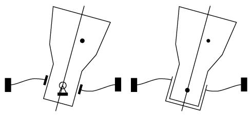
**Fig. 2.** A rigid body on an elastic plate. The body has a fixed point.
