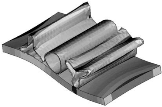
Fig. 3. Example of a high-frequency natural mode: vibrations of the substrate and nanotubes.
