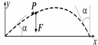
$$\begin{cases} V_x = V_0 \cos \alpha - \frac{F}{m}t, \\ V_y = V_0 \sin \alpha - \frac{P}{m}t, \\ x = V_0 \cos \alpha t - \frac{F}{m} \frac{t^2}{2}, \\ y = V_0 \sin \alpha t - \frac{P}{m} \frac{t^2}{2} \end{cases}$$
